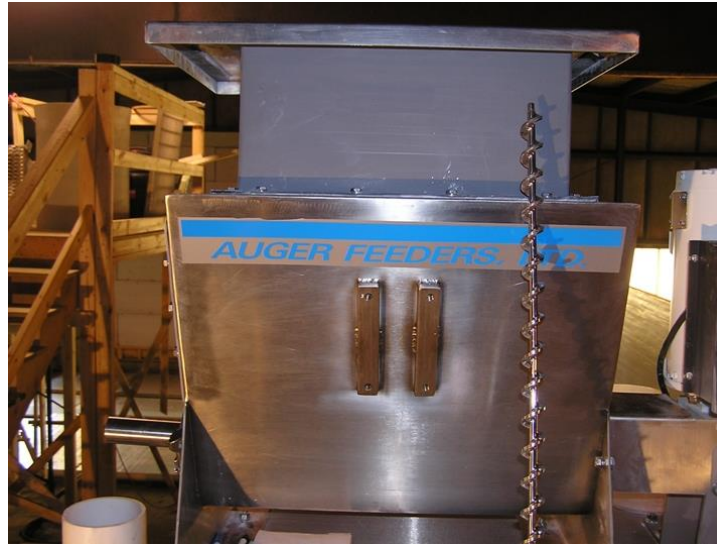
Figure 6: Photograph Showing Variable-speed Auger Feeder
