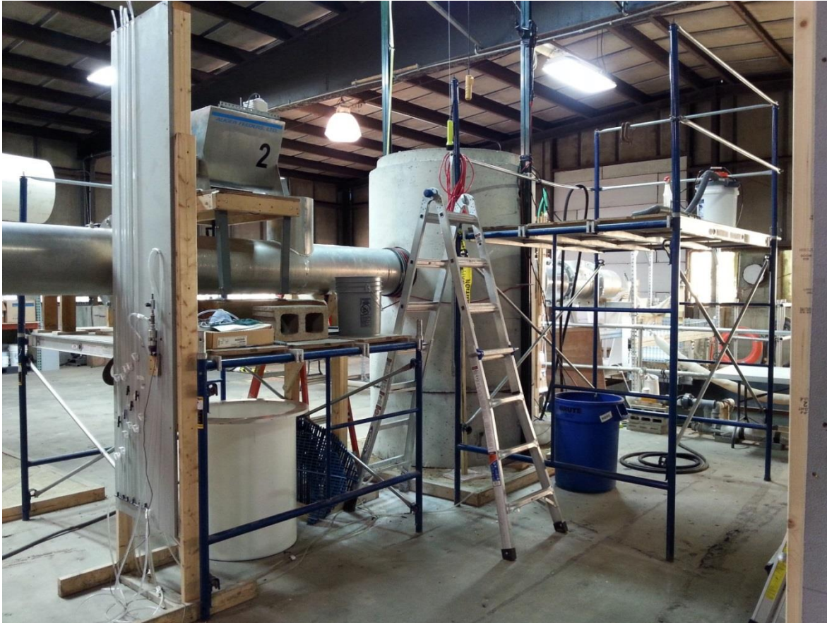
Figure 2: HS 4 Test Unit Installed in Alden Flow Loop
