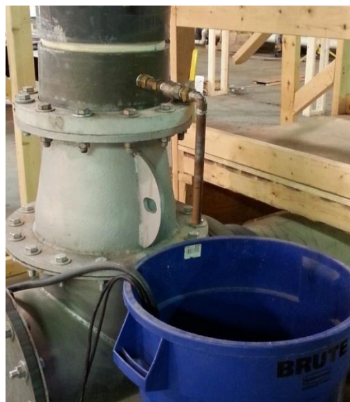
Figure 7: Photograph Showing the Background Isokinetic Sampler
