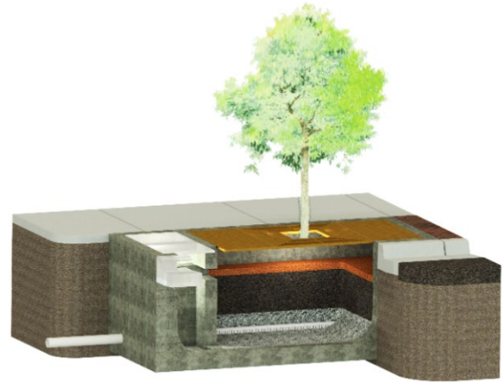
Bypass Weir Model
