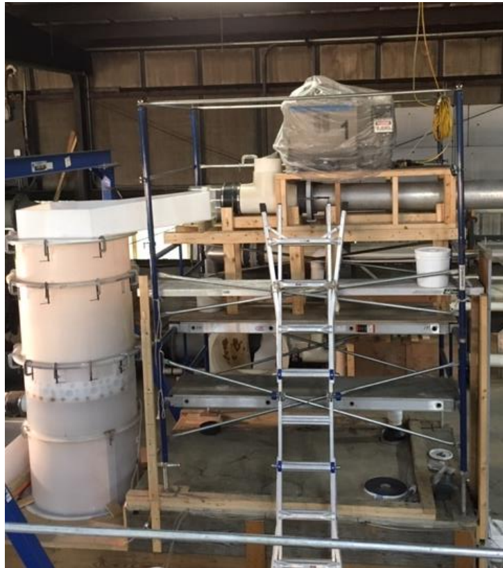
Figure 4 Hydroworks HydroFilter Test Set-up
