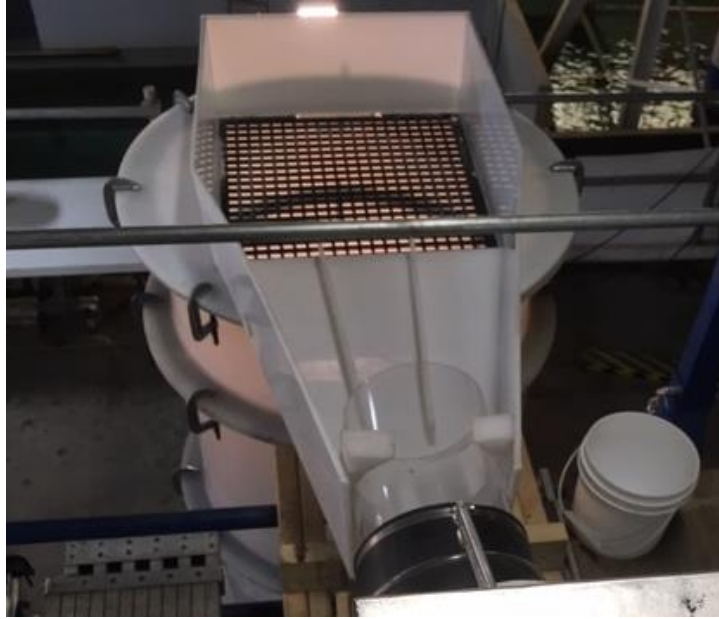
Figure 5 Test Loop Grated Inlet
