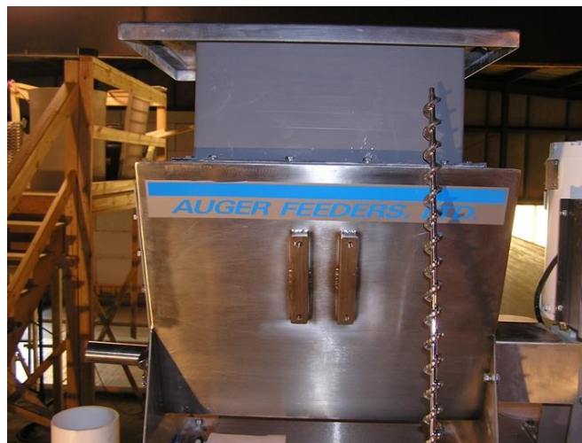
Figure 10 Photograph Showing Variable-Speed Auger Feeder
