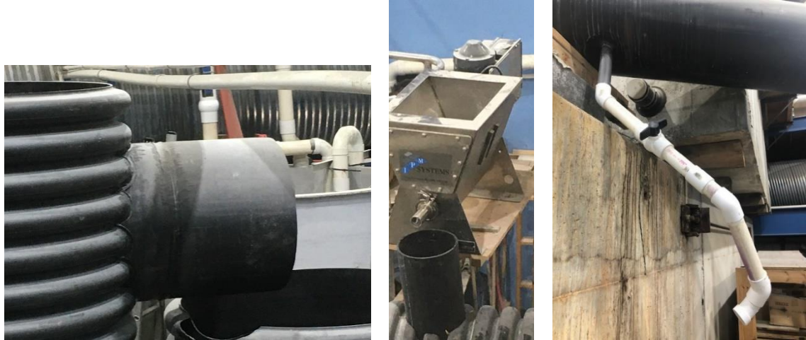
Figure 3 Barracuda MAX Test Unit Effluent Sampling Area, Sediment Dosing Port, and Background Sampling Area
