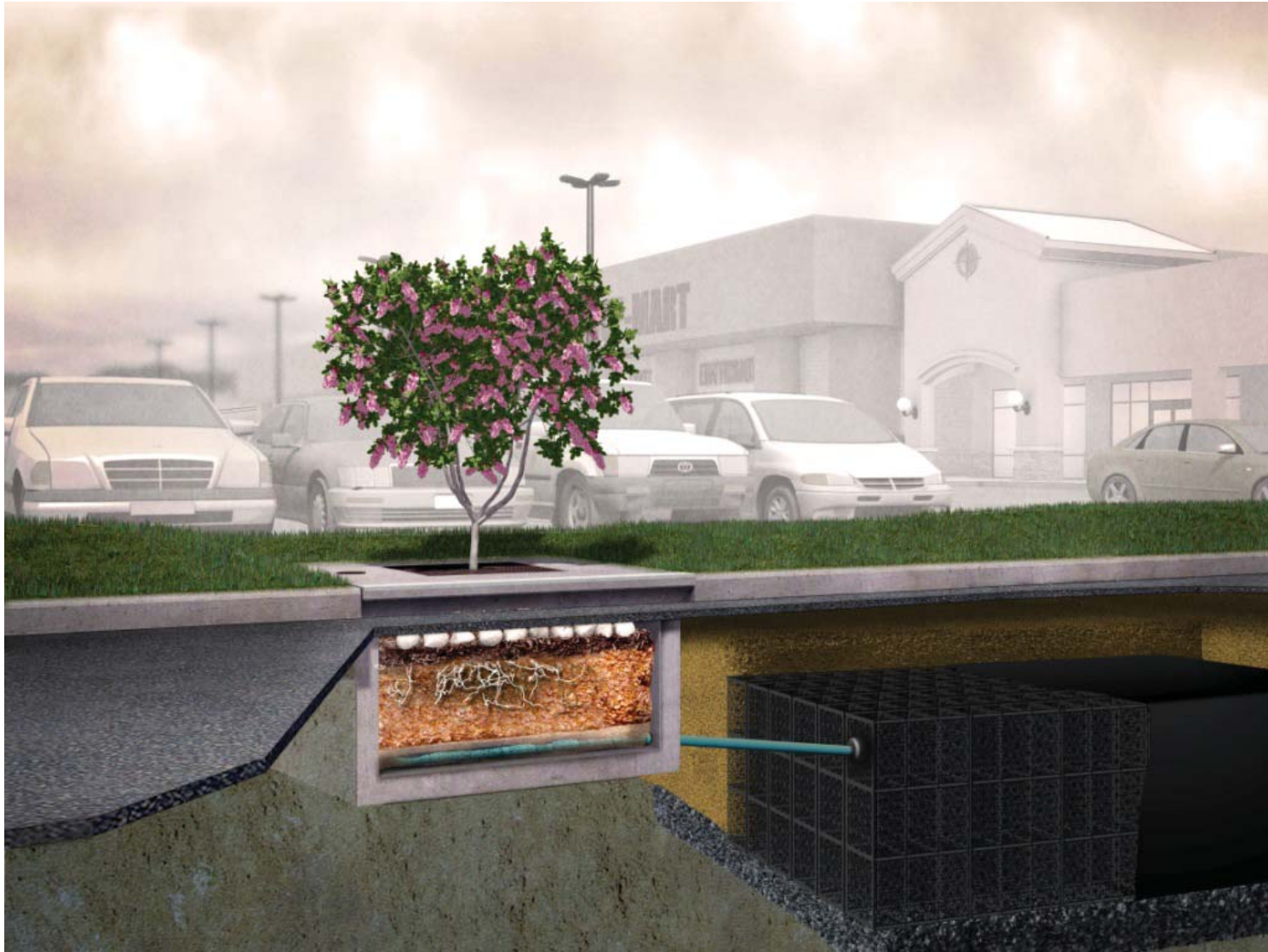
Figure A-2. Filterra® system discharging to a rain tank.
