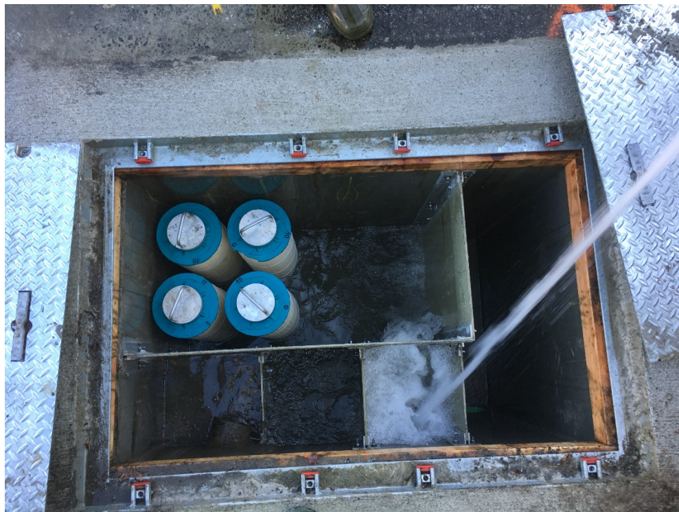
Figure 11. Water Being Discharged into the Tacoma Dome Test System at 34 gpm, the Design Flow Rate.
