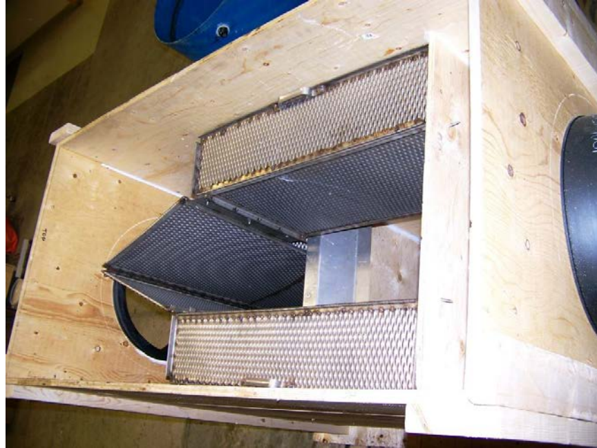
Figure 6 Debris Separating Baffle Box in Plywood Vault
