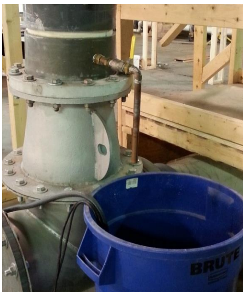
Figure 8 Photograph Showing the Background Isokinetic Sampler
