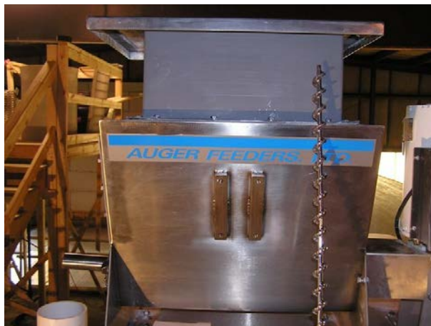
Figure 7 Photograph Showing Variable-Speed Auger Feeder
