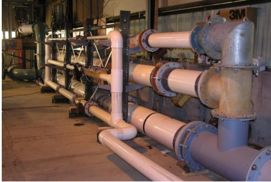
Figure 5 Photograph Showing Laboratory Flow Meters
