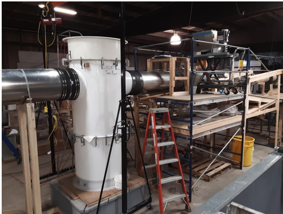
Figure 3 HydroDome HD 3 Test Unit Installed in Alden Test Loop
