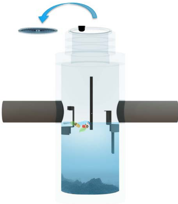
Remove Access Hatches Set Up Vacuum Truck to Clean the Sump Chamber.
