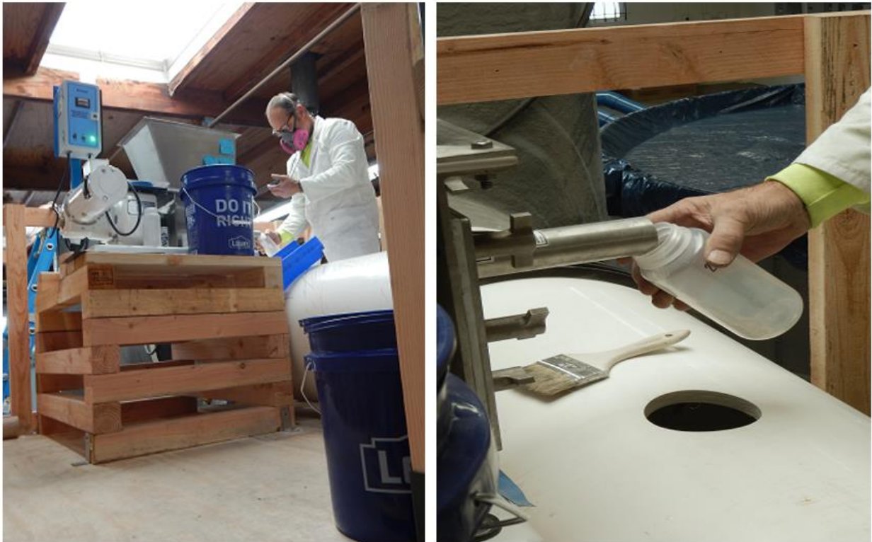
Figure 8 Sediment Addition Point
