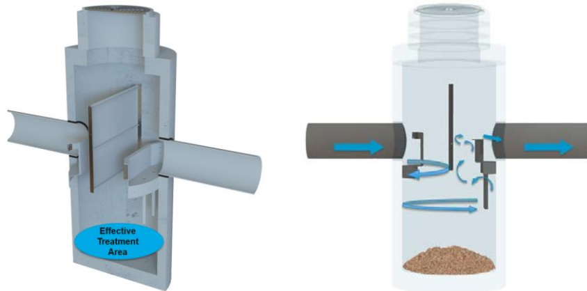
Figure 3 Effective Treatment Area and Flow Path Diagram
