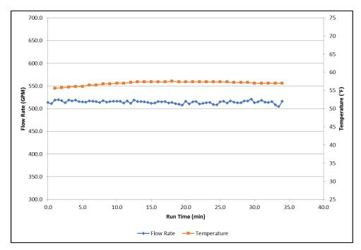
Figure 14 Water Flow and Temperature - 100% MTFR
