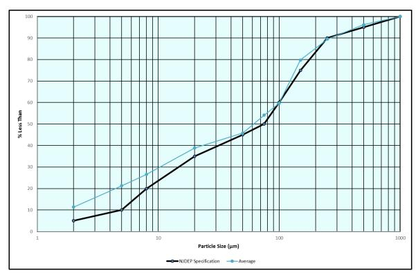
Figure 8 Average Particle Size Distribution of 1-1000 μm Test Sediment
