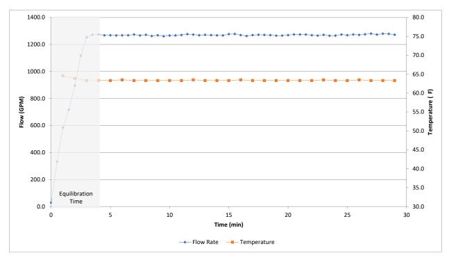
Figure 19 Water Flow and Temperature - Scour Test
