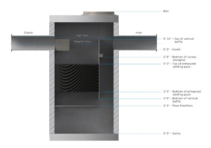
Figure 3 4-Foot System with Component Elevations
