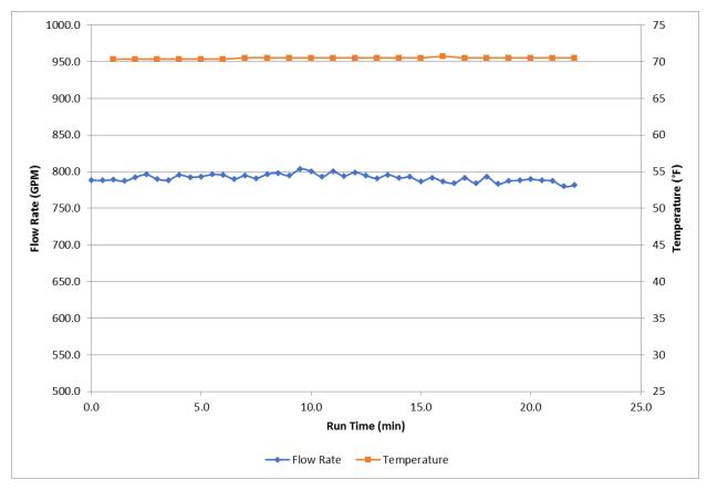
Figure 17 Water Flow and Temperature - 154% MTFR
