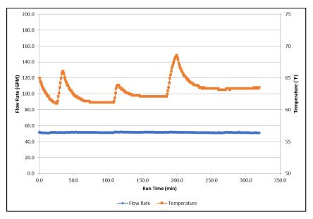
Figure 10 Water Flow and Temperature - 10% MTFR
