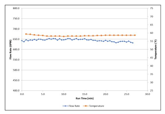
Figure 15 Water Flow and Temperature - 125% MTFR
