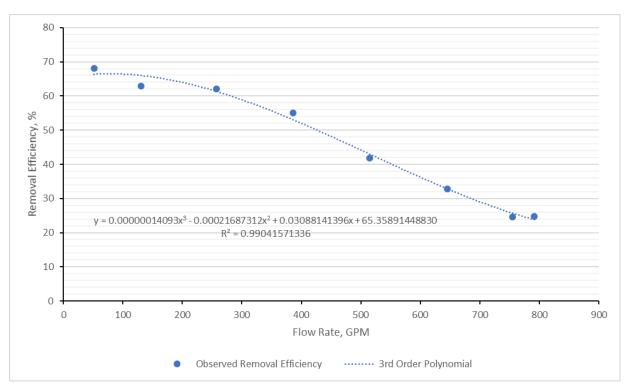
Figure 18 StormSettler® Removal Efficiency Curve
