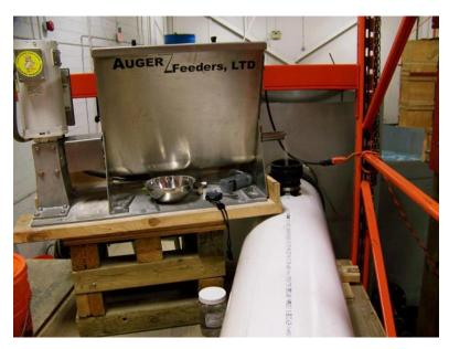
Figure 7 Sediment Auger Feeder
