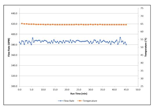
Figure 13 Water Flow and Temperature - 75% MTFR
