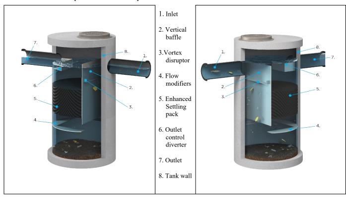
Figure 1 StormSettler Low Flow Operation
