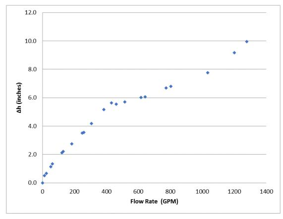
Figure 20 StormSettler Head Loss
